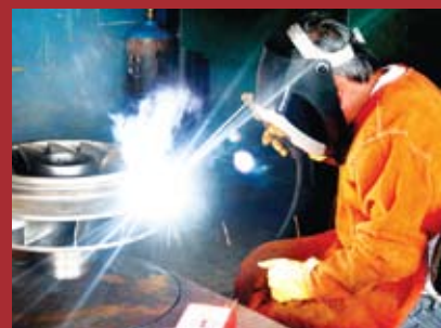
THE MASTER AT WORK. Newly certified Efren Eddio sparks up a Francis runner in this display of superb welding skills.
