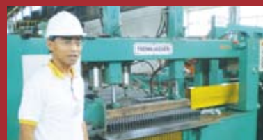
Reuel Velasco earlier inspected the steel grating cutting stage of Ishida's manufacturing process flow.
